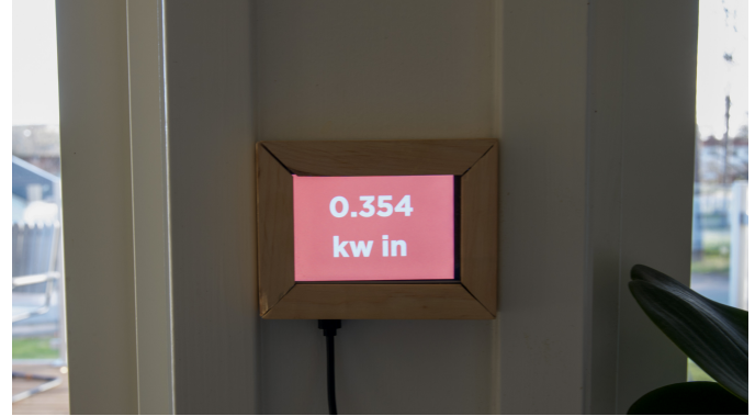
Fig. 2. Always-On Display showing a total consumption of 0.354 kW in a household. The red background indicates that the house is consuming/buying electricity from the grid
