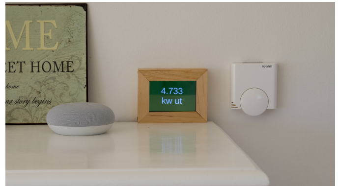
Fig. 3. Always-On Display showing a total consumption of 4.733 kW in a household. The green background indicates that the house has surplus energy and is selling electricity to the grid
