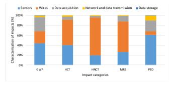
Fig. 4. Environmental and resource impacts for the KTH live-in lab case.
