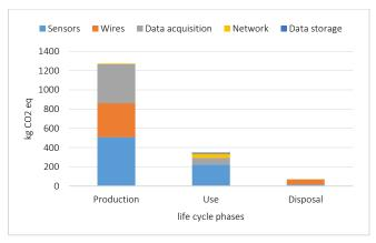
Fig. 5. Global warming potential for different life cycle phases for the KTH live-in lab case.
